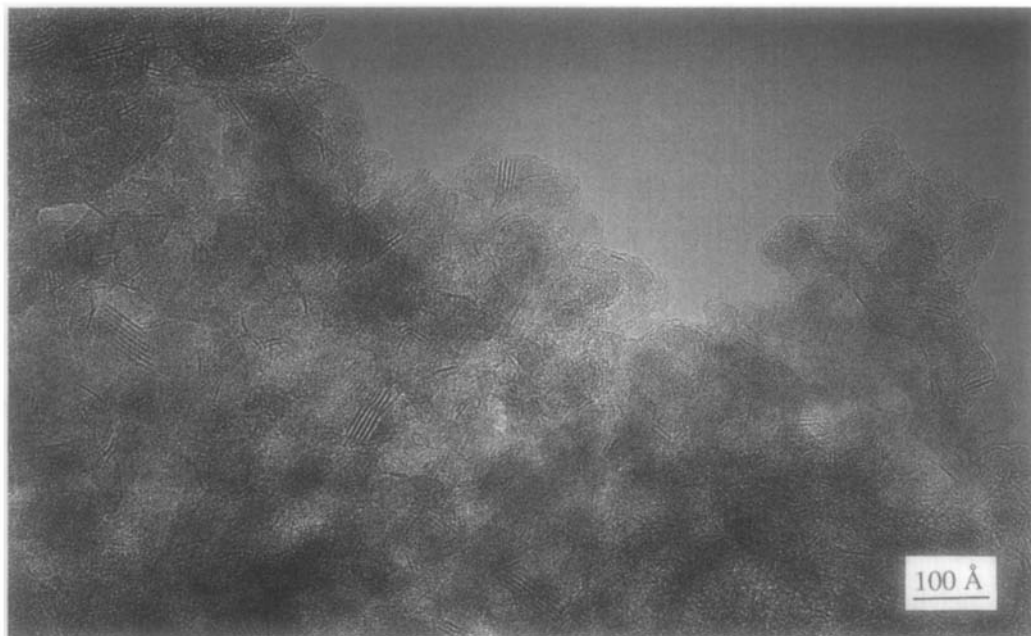
FIG. 2. A high resolution electron micrograph of a sulfided industrial (Katalco) HDS catalyst which consisted of \text{CoO-MoO}_3 supported on alumina. Note the slabs of \text{MoS}_2 dispersed on the \text{Al}_2\text{O}_3 indicated by the short dark 6.15 Å lattice fringes.
